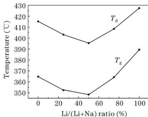
Fig. 3. Dependences of  $T_g$  and  $T_d$  on Li/(Li+Na) ratio.
