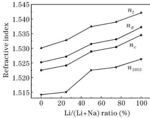
Fig. 1. Dependence of refractive index on Li/(Li+Na) molar ratio.
