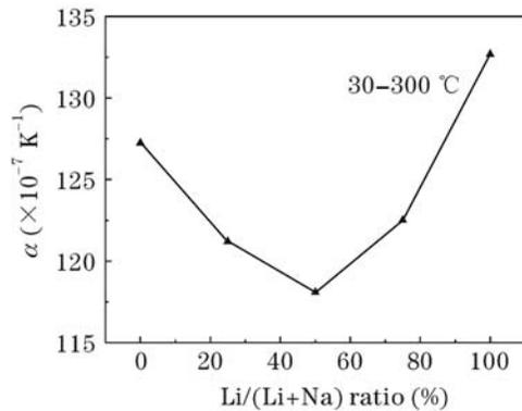
Fig. 2. Dependence of  $\alpha$  on Li/(Li+Na) ratio.
