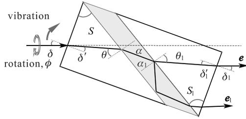
Fig. 2. Schematic diagram showing the passage of a beam of light transmitted through a spinning Glan-Thompson-type prism.  $\delta$  is the vibration angle of the prism, and it together with the gap between constituent prisms are exaggerated for clarity.
