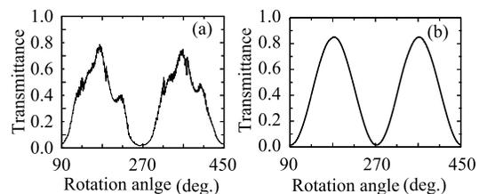
Fig. 1. Measured transmission versus the rotation angle for spinning (a) air-spaced and (b) cemented Glan-Thompson-type (with the gap refractive index  $n_G=1.54$ ) prisms for 650-nm linearly polarized light. The thickness of each prism gap  $h$  is 0.02 mm.
