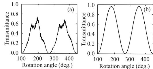
Fig. 4. Numerical transmission versus the rotation angle for the (a) air-spaced and (b) cemented ( $n_G=1.54$ ) Glan-Thompson-type prisms, with  $h=0.02$  mm and  $\lambda=650$  nm. The cut angle is  $38.07^\circ$  for the former and  $69.5^\circ$  for the latter.
