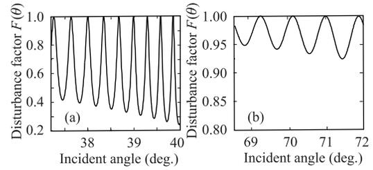
Fig. 3. Numerical disturbance factor as a function of the incident angle  $\theta$  at the gap for the (a) air-spaced and (b) cemented ( $n_G=1.54$ ) Glan-Thompson-type prisms, with  $h=0.02$  mm and  $\lambda=650$  nm.
