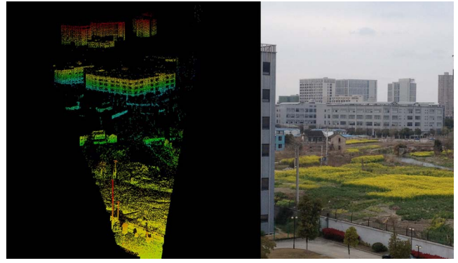
Fig. 9. Front view of point-cloud of the three-dimensional imaging (on the left), and a photograph of the same place (on the right).
